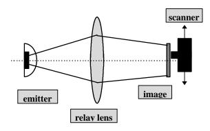
Figure 9. Apparent Source Size Measurement
