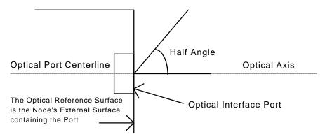
Figure 3. Optical Port Geometry
