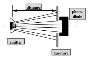
Figure 10. IEC 60825-1 AEL Classification Power Measurement
