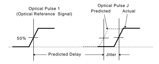
Figure 7. Pulse Delay and Jitter Definitions
