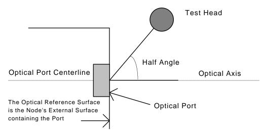
Figure 4. Optical Port Angle Measurement Geometry
