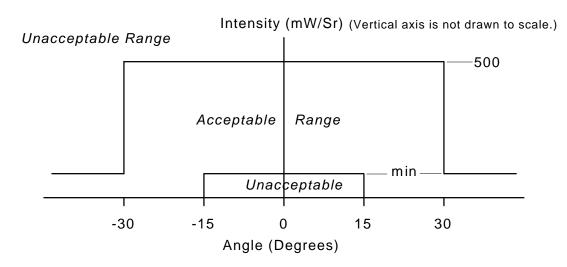
Figure 5. Acceptable Optical Output Intensity Range
